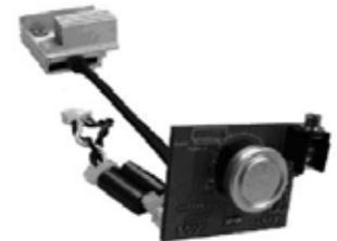
Thermostatic Controlled Heater Kit for the Effio V Platform cameras.
