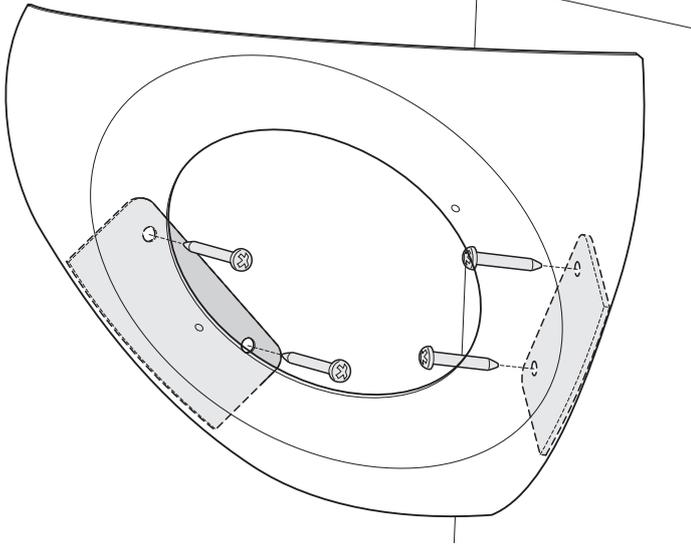
Position the corner mount in the required position. Use screws and wall plugs (as appropriate to the wall surfaces) to fix the corner mount in position. Access to the screw positions is gained through the open front aperture of the corner mount.
