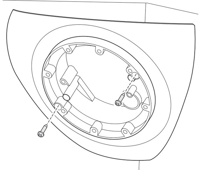
Use the supplied screws to secure the dome enclosure to the corner mount. Continue reassembling, wiring and focussing the dome and its camera according to the supplied instruction sheets.
