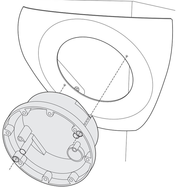
Place the dome enclosure (remove the outer ring, if fitted) within the front aperture of the corner mount. Align the two enclosure mounting holes indicated, with the corresponding threaded holes within the front face of the corner mount.
