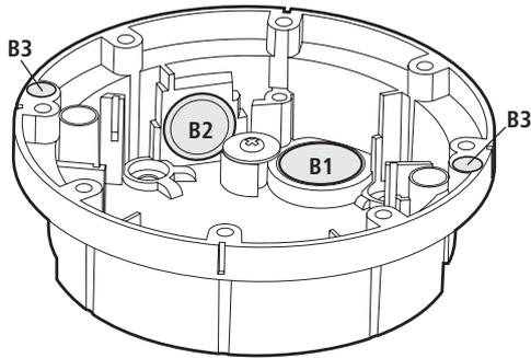
With the camera assembly removed, decide which entry point will be used either (B1) the 3/4" conduit entry or (B2) the 1/2" side conduit entry and remove the appropriate plug. Carefully drill (or tap out) the mounting holes (B3).
